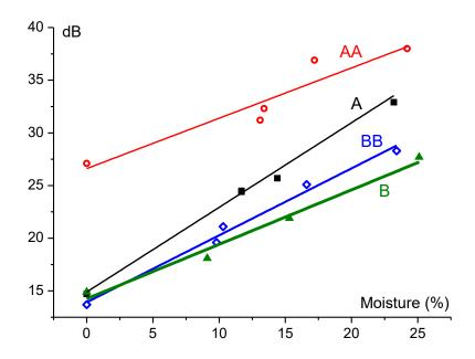
Figure 1. Relative attenuation by the charcoal layer against the moisture
