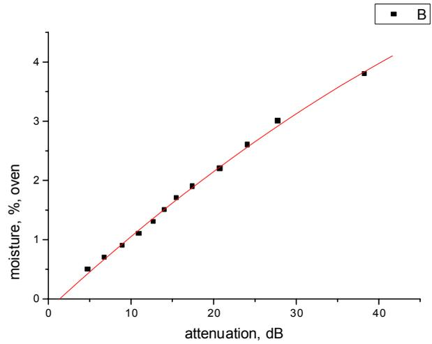
**Fig. 7** Dependence of attenuation on moisture for salt NaCl. The measurements were conducted in the rectangular waveguide of 23-10 mms at 10,5 HHz, mass is 25 g.
