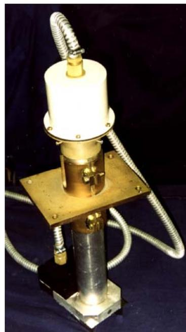
**Fig. 9. The equipment for research of metrology parameters of the resonator two-parameter method.**
