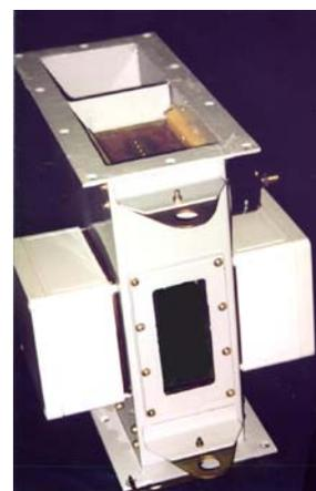
**Fig. 4. Dependence of attenuation on moisture in on-line microwave sensor and its outward.**
