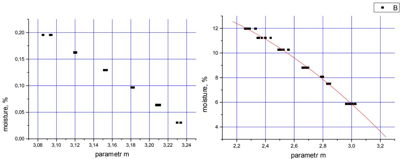
Fig. 10 The results of tests for sugar (on the left) and fish flour (on the right). For sugar SD=0.0031 % abs., R=0.9977; for a fish flour SD=0.19 % abs, R=0.992.
