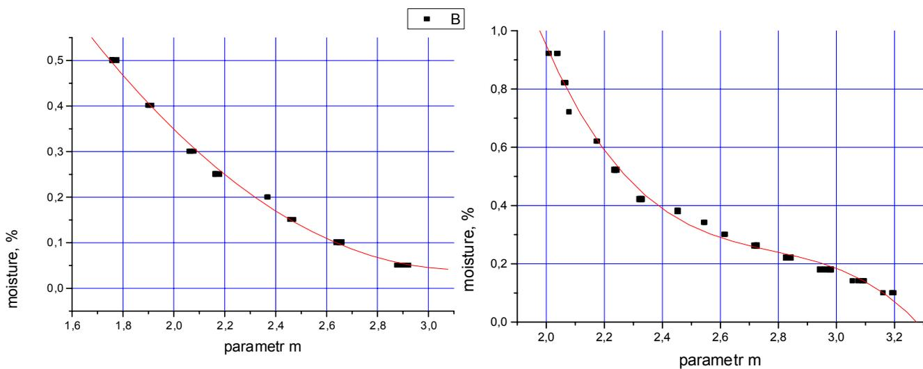
Fig. 11. The results of researches of sulphate of ammonium (on the left) and NaCl (on the right). For sulphate of ammonium SD=0.011 % abs., R = 0.995; for NaCl SD=0.025 % abs., R=0.99.
