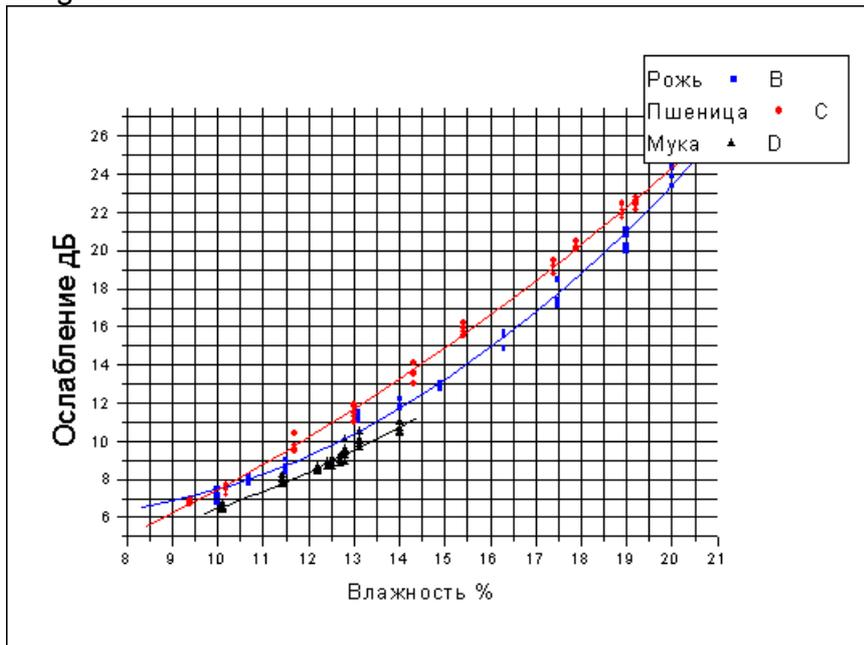
**Fig.1. Dependences of microwave attenuation on grain wheat ,rye and wheat flour moisture at 10 GHz frequency.**
